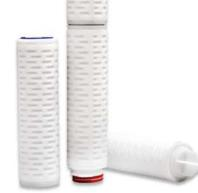
Nupore PP (CFPP) cartridge filters are available in a wide range of pore size ranging from  $0.2\mu$ m to  $50\mu$ m and are especially designed and developed for high particle retention, dirt holding and pre-to-final filtration applications i.e. aqueous filtration and venting application.
